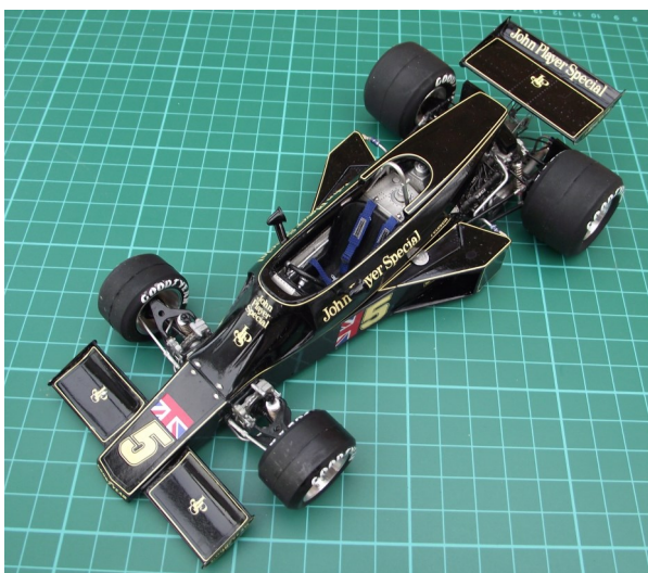
Early season Lotus 77 (1:20) above with the chunky outboard brake sub-frames compared to the later season, (1:12) right, and the more elegant outboard braking set
